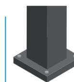
**POTEAU TUBULAIRE AVEC PLATINE DE FIXATION AU SOL DÉBORDANTE**
